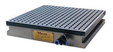
Chuck surface grid for 10 \* 10mm dense style, effectively increase the adsorption area and vacuum space. Suction cup material for tempered steel, wear resistance is stronger. Lattice can be tapped and punched (diameter 8MM, depth of 20MM or less), can be used for fixing or positioning.
