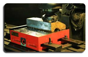
The super strong magnetic holding force is from the combination of square or strip magnetic units. The units distributes intensively, powerful strength of magnetic fields. It can release the internal stress of workpiece in machining, get the high precision product
