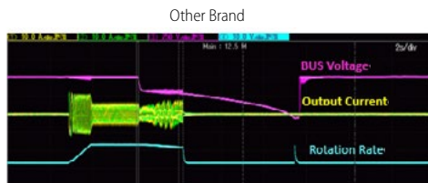
At power failure, unit runs for 3s, UV alarm motor stops freely
