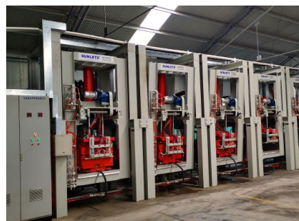
WC Pan High Pressure Casting 坐便器高压成型线
