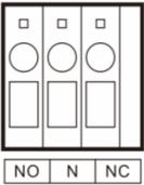
This contact automatically starts the generator and charges the battery bank. Under normal conditions, this terminal is NC-N point closed, NO-N point open. When the battery voltage reaches the low voltage point, the relay coil is energized, and NO-N point now is closed and NC-N point now is open.
