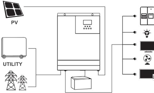
**Photovoltaic Modules (PV):** convert light energy into DC power, charge the battery through the solar inverter charger, or directly reverse into alternating current to power the load.
