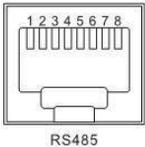
This port is an RS485 communication port ; Communication is an optional function, which is not available in the standard machine.
