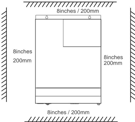
**Please Note:** While the Solar inverter has fans for cooling, this installation location optimal for natural convection cooling will improve the overall efficiency
