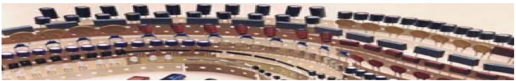
Component Spacing for 12.7 (0.500) Pitch Tape
