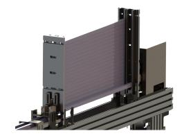
High storage capacity (purple area above): The maximum material storage capacity is 40 tubes, which effectively reduces the frequency of operator refilling and liberates labor
