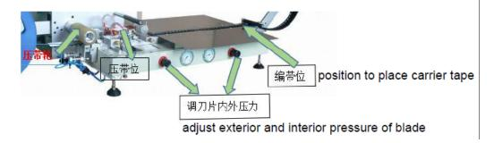
**Feeding:** put on empty carrier tape, which to be used to pack components
