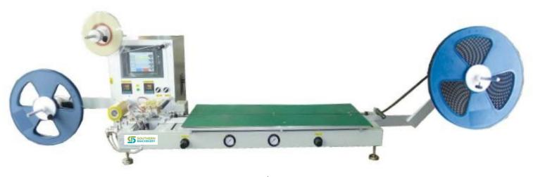
use wrench to adjust nuts of four support feet, keep platform surface to horizontality, as the first condition of calibration.
