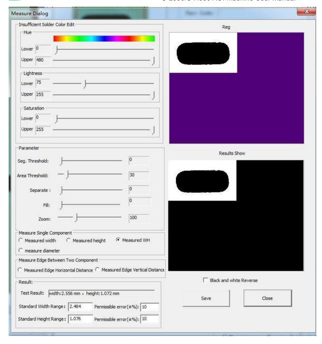
After setting or adjusting the registration information parameters, the user should press the application button to save. If the component has been entered, the result will be stored in the library file. Otherwise, the result will be stored in the registration information of the component. If the inspection frame has multiple groups, the user can choose to update all groups simultaneously with the modified information.
