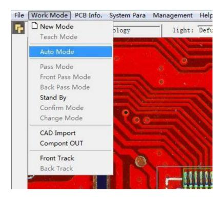
In addition to several main working modes, there is a pass mode for the on-line machine. In this mode, the boards on the track directly pass through the on-line machine. Only the number of boards is counted, and no inspection will be carried out. In other words, the on-line machine serves as a inspection conveyor.
