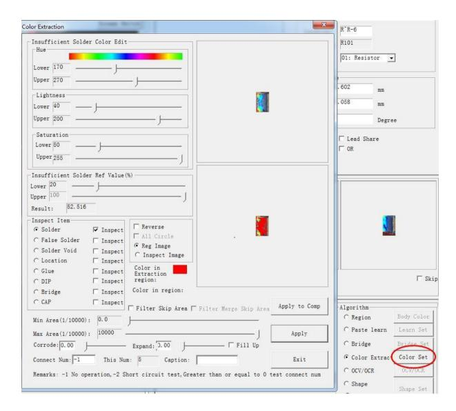
Compared with the single inspection frame of other algorithms which contains only one standard (different standards can be expanded only by adding groups), the single inspection frame for color extraction in this system
