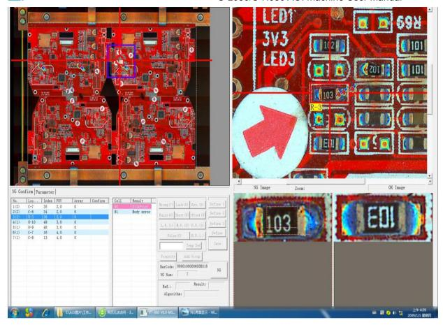
If the current PCB inspection has an inspection frame determined as NG, the NG result display interface will pop up after the inspection is completed for comparison and confirmation by users.
