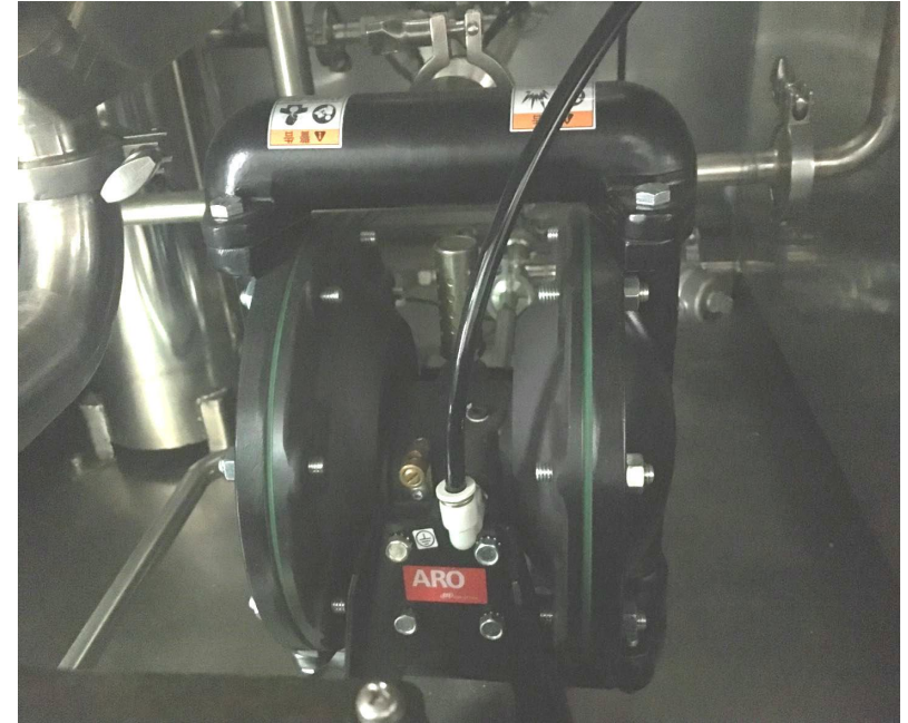
Ingersoll Rand air pump for liquid and water automatically add and discharge
