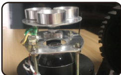
2. Loosen the screws and take out the heat sink
