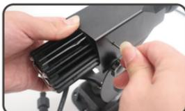
2. Use the hexagon wrench to loosen screw; then take out the heat sink
