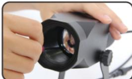
2. Rotate the optical lens by anticlockwise
