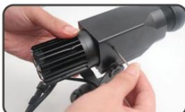
5. Install the heat sink into the projector and fasten the screw
