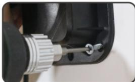
1. install screws to fix the projector
