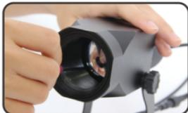
2. Rotate the optical lens by anticlockwise
