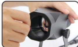
3. Rotate the optical lens by clockwise
