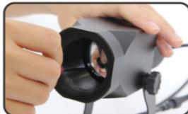
2. Rotate the optical lens by anticlockwise
