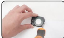
3. Loosen the screws on the gobo bracket; take out the old gobo
