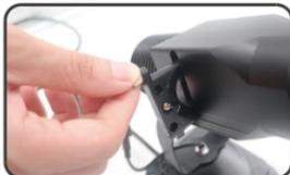
2. Loosen the screw on the side, take out the gobo bracket
