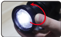
3.Ajust the image definition by rotating the zoom lens
