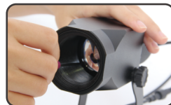
2.Rotate the optical lens by anticlockwise Effect: Image Bigger
