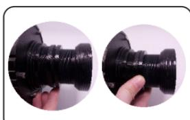
1. Screw out the ring on the front lens to adjust image
