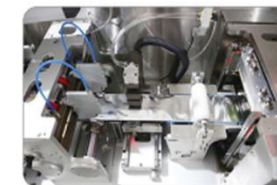
废边分切及往复易撕口部分 Both sides cutting and easy tear making
